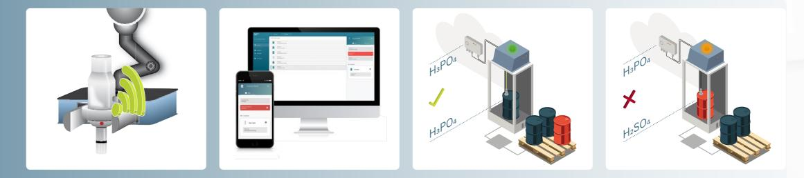
Automatic chemical detection (RFID): chemical, concentration, supplier, container expiration date, etc. Automatic and complete traceability: reports when each drum with the specific chemical and batch was emptied Pump release only with matching chemical
